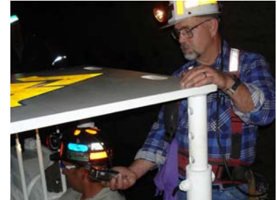
Larry Wine , district inspector in the Oak Hill region, is shown here underground performing the diluted emission test at the operator's station of the Mini-Trac diesel forklift.
