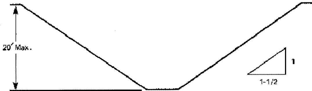
Figure 1. Excavations Made in Type C Soil All simple slope excavations 20 feet or less in depth shall have a maximum allowable slope of 1 1/2:1.
